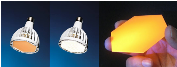
Figure 5.8: Picture of a remote phosphor converted white LED for general lighting using commercial quantum dots (from QD Vision). [142;143]
