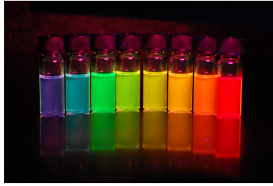
Figure 1.1: A series of dilute suspensions of CdSe QDs in toluene, with diameters ranging from \approx 2 to 5 nm. (QDs by S. Abé, picture by I. Moreels)
