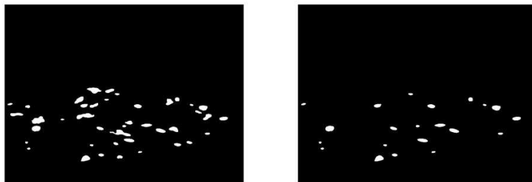
Figure 2 - Outlined original image before (left) and after (right) the application of the filter based on circularity and convexity.
