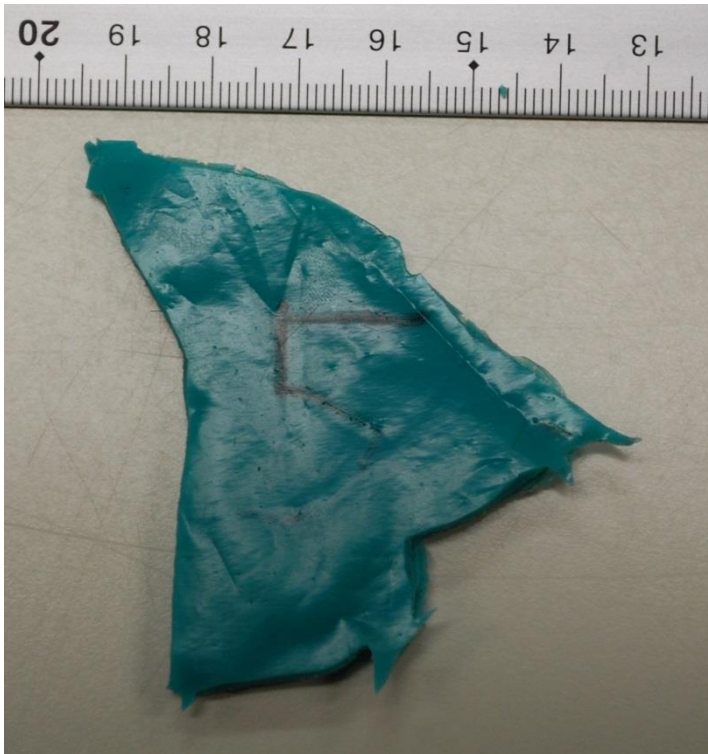
Figure 5. Picture perpendicular to the surface of a wound silicone cast with a metric scale to be processed with the ImageJ 1 program to calculate the area and circumference of the cast.
