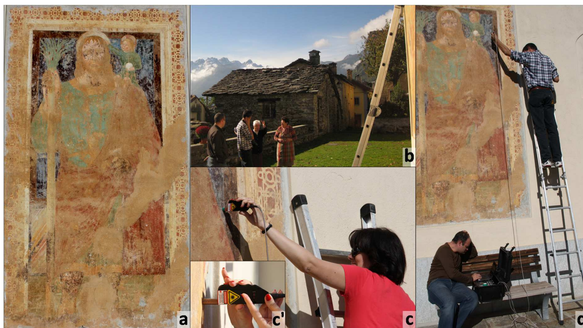
Figure 3.5 Evaluation of the portable Raman spectrometer by analysing the pigments of the mediaeval wall painting of S. Cristoforo at the church of Pianazzola (a). During the analysis the research was explained to the inhabitants of the village (b). During the analysis the probehead was manually positioned (c-d) and the sunlight was blocked out by sliding a copper tube over the objective lens (c').
