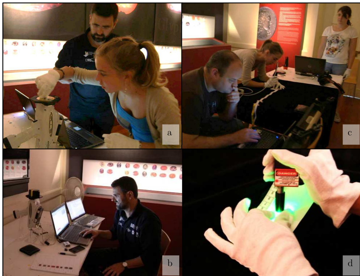
Figure 5.2 Overview of the experimental set-up during the analysis of the glyptics. a-b: Handheld XRF experiments (hXRF). c-d: portable Raman spectroscopy.
