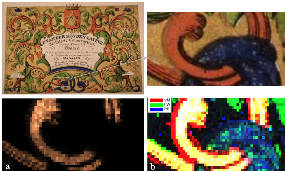
Figure 8.5 (a) Map of a single variable illustrating the distribution of the characteristic Raman band of vermilion ( 262\text{ cm}^{-1} ); (b) Map of a multiple variables illustrating the distribution of the characteristic Raman band of vermilion ( 262\text{ cm}^{-1} ), lead white ( 1050\text{ cm}^{-1} ) and Prussian blue ( 536\text{ cm}^{-1} ). Bands in both images are extracted with the ENet extraction function.
