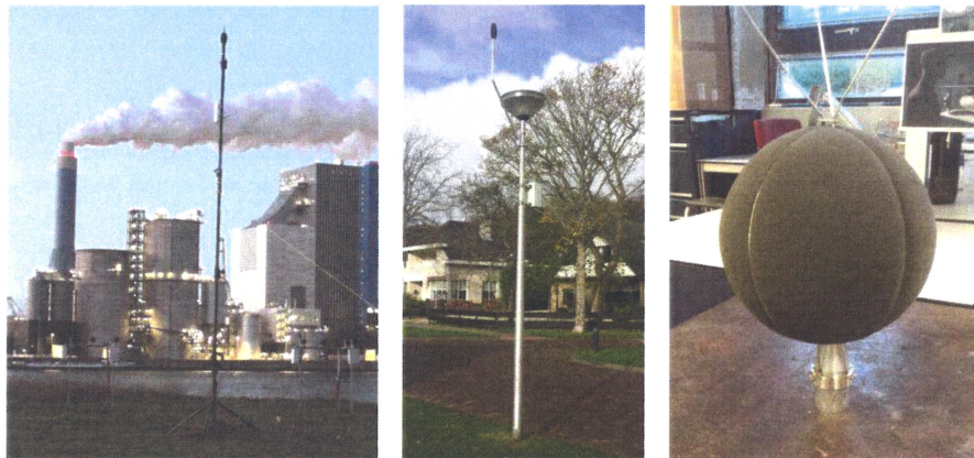
Figure 3 – An IA microphone (left), a RA microphone (middle), the 18cm applied windscreen (right).
