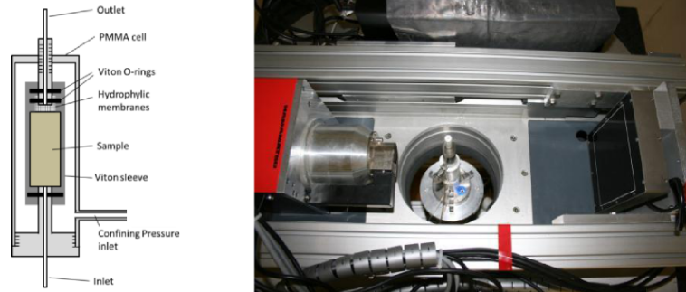
Figure 7.2: A custom-built PMMA confining-pressure flowcell (left) allows the visualization of fluid flow in stone samples with a diameter of 6 mm and a height between 15 and 20 mm. UGCT's EMCT scanner (right) was built in collaboration with XRE. The flow cell is mounted on a stand which moves into the scanner from below. The gantry (with the source and detector mounted on it) rotates around the sample, while the sample remains static.
