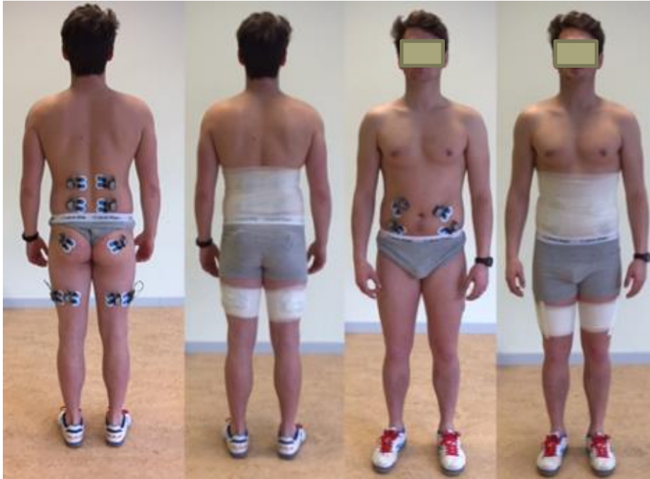
Figure 2. Electrode and amplifier placement for MVC- and sprint trial sEMG data collection.
