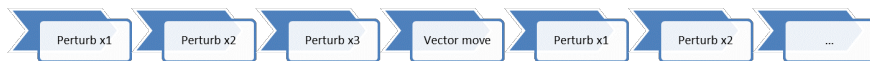
Figure B.6 One-at-a-Time move of Hooke & Jeeves Method of a three variable problem
