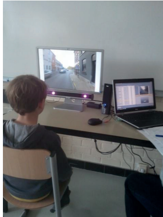
Figure 2. Experimental set up. Red dots on the eye-tracker are infra-red lights, and cannot be seen by the participant
