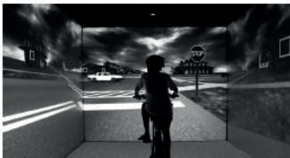
Figure 23. Picture from the bicycle simulator at the University of Iowa. Visual angles are correct from the rider's viewpoint (Nikolas et al., 2016).
