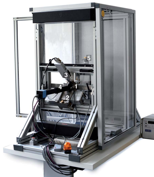
Fig. 3 Compact (3D) micro-XRF spectrometer. (1) gauge head; (2) X-ray tube; (3) silicon drift detector; (4) microscope with camera; and (5) encapsulated positioning stage.
