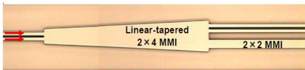
Figure 1.7: Schematic for the novel 90^\circ optical hybrid consisting of a 2 \times 4 MMI coupler and a 2 \times 2 MMI coupler [47].
