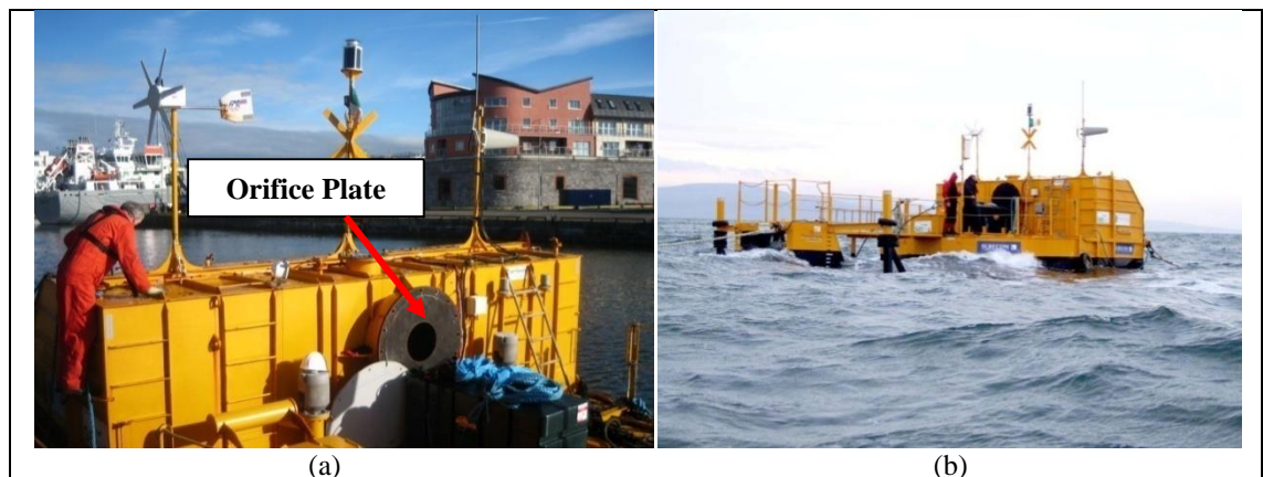
Figure 1.4. (a) Phase 3 OE Buoy with orifice plate to model PTO and (b) on site in Galway Bay.
