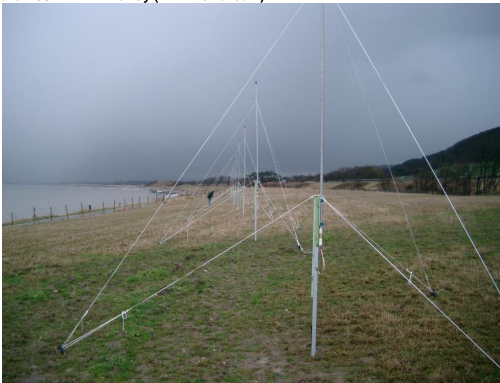
Figure 2.34 WERA RX array ( www.helzel.com ) Ocean Radar Theory
