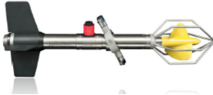
Figure 2.41 Propeller type current meter (Source: www.Valeport.co.uk )
