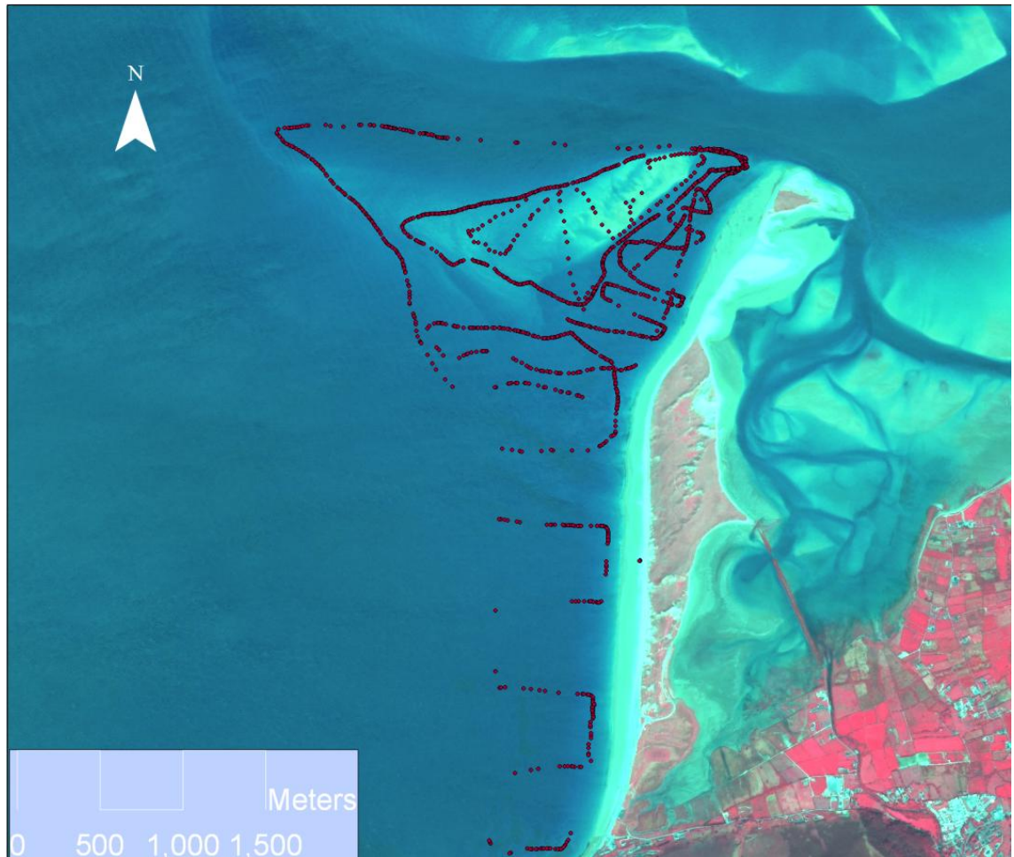
Figure 4.34 Bathymetry Survey of Rossbeigh March 2013
