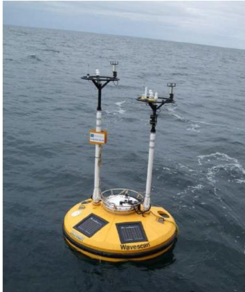
Figure 2.29 Fugro Wave scan PRH buoy (Courtesy Marine Institute)
