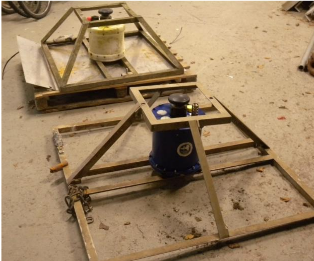
Figure 2.30 Valeport Bottom Mounted Pressure Sensor Wave Gauges
