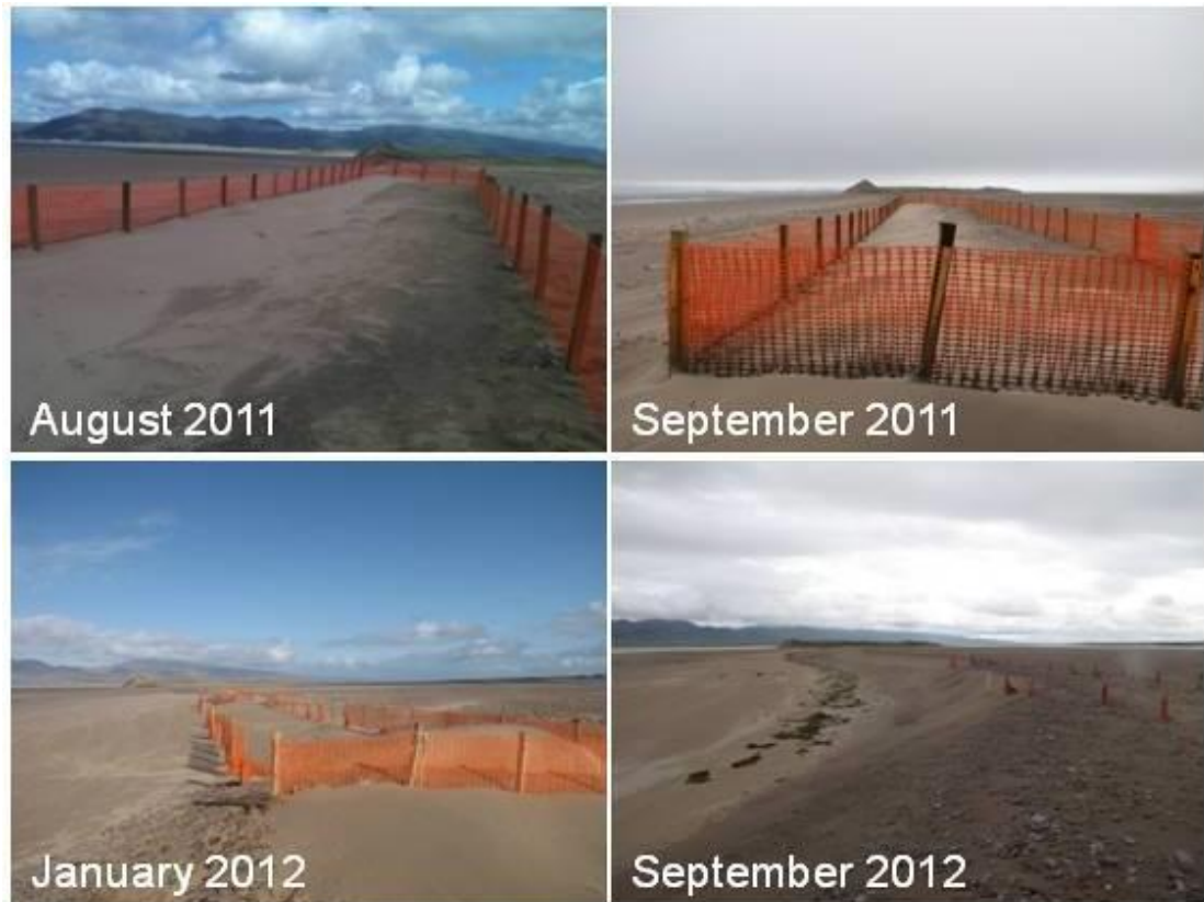
Figure 7.14 Aeolian fencing trials on Rossbeigh
