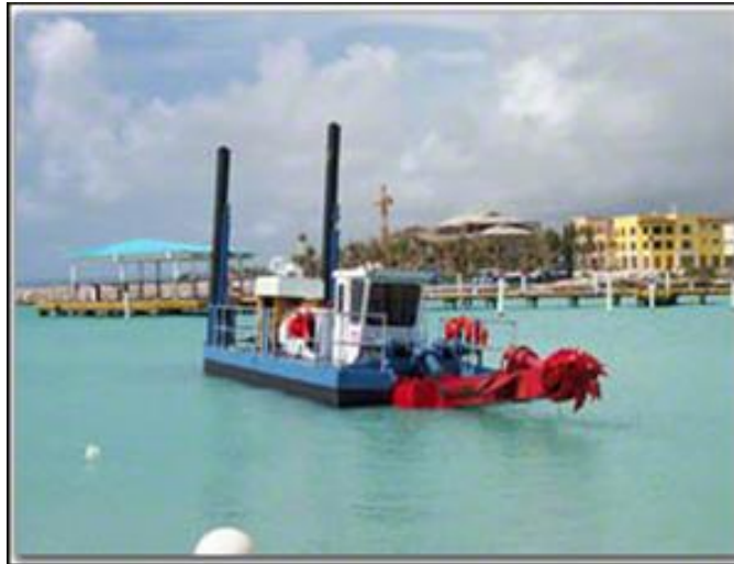
Figure 7.13 Cutter suction dredger suitable for Rossbeigh beach nourishment
