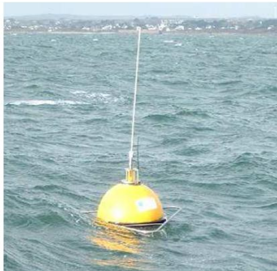
Figure 2.28 Waverider buoy (Courtesy Of Marine Institute)
