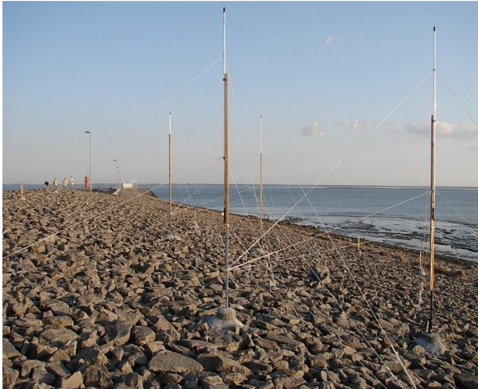
Figure 2.33 WERA TX array ( www.helzel.com )
