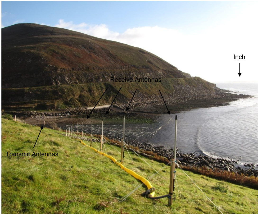
Figure 5.3 North Site radar station setup looking toward Inch
