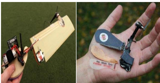
Figure 1: Example of past developed UAVs. Left: Lockheed Martin SAMARAI [1]. Right: University of Maryland Monocopter [2]
