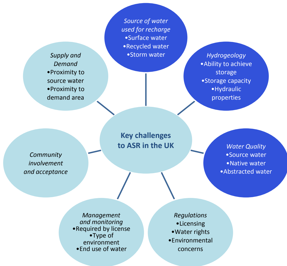
Figure 2.1: Summary of the key challenges to ASR in the UK. The Dark blue bubbles represent the operational and hydrological challenges and pale blue bubbles represent the non-technical constraints
