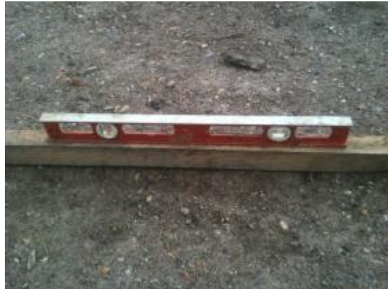
Figure 4-22 Equipment used in levelling the soil surface
