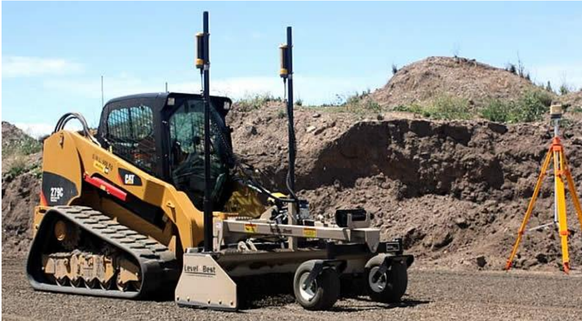
Figure 4-1 Laser-level grading equipment used for grading and re-grading of 'flat' LBWWT systems (ATI Corp., 2014)
