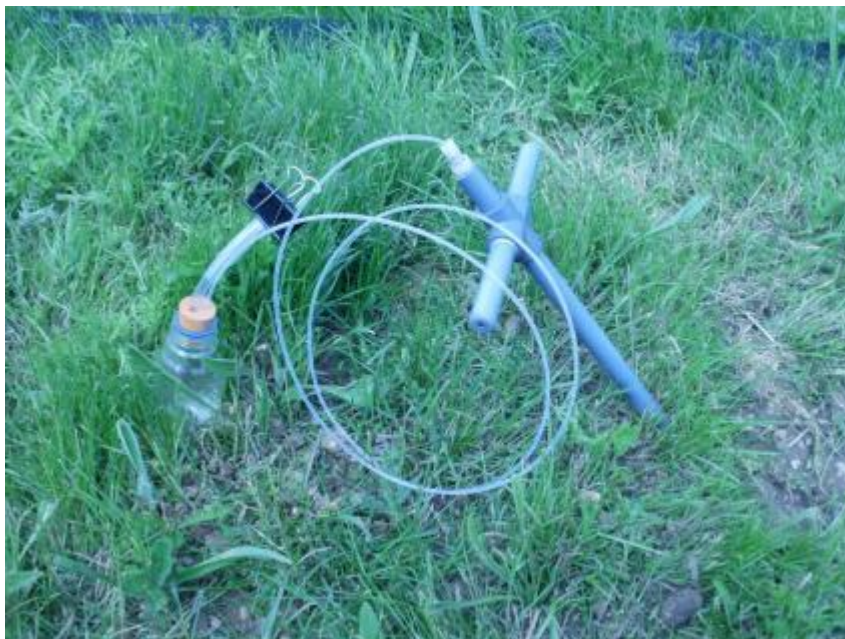
Figure 4-27 Fully installed suction cup
