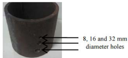
Figure 9: Forged steel round test cylinder.
