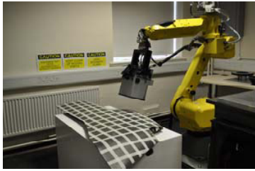
Figure 6: The robotic arm presenting the thermoscope at multiple regular positions and angle to capture images of a large component.
