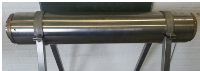
Fig. 2. Custom-made core holder for large-scale core-flooding experiments.
