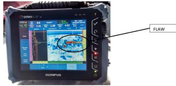
Fig. 5. Result of experiment and analysis of sample showing flaw characteristics.
