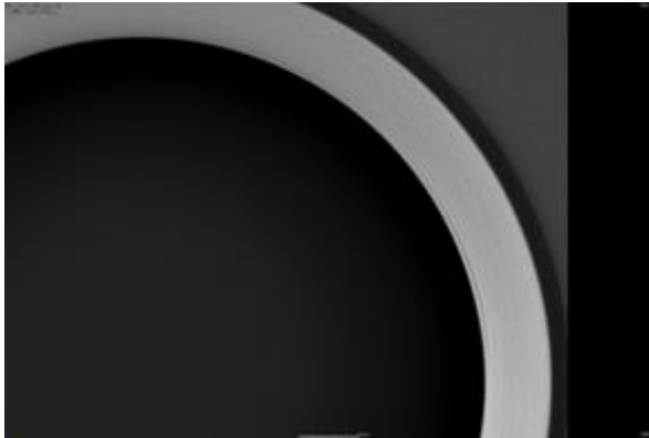
Fig. 10. Slice through the volumetric model acquired by CT scanning; the delamination on the inner side can clearly be detected
