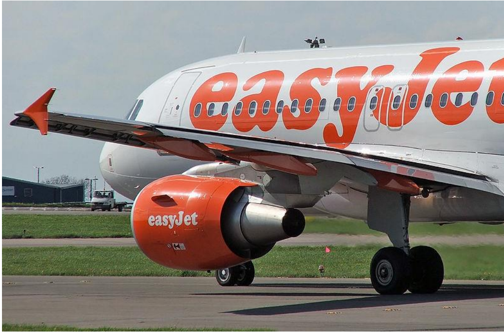
FIGURE 3.21: CFM56 ENGINE ON AIRBUS A320 AIRCRAFT (COLLINS 2006)
