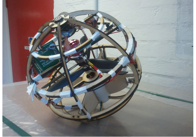
Fig. 14. The completed flight ready spherical UAV.
