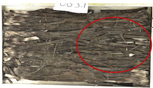
Fig. 7. First ply of plate GO3 in the mould; the red circle indicates a lower tow density. (For interpretation of the references to colour in this figure legend, the reader is referred to the web version of this article.)
