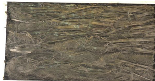
Fig. 2. One ply of recycled carbon fibres incorporating fluffy tows ( 150 \times 280 \text{ mm}^2 ).
