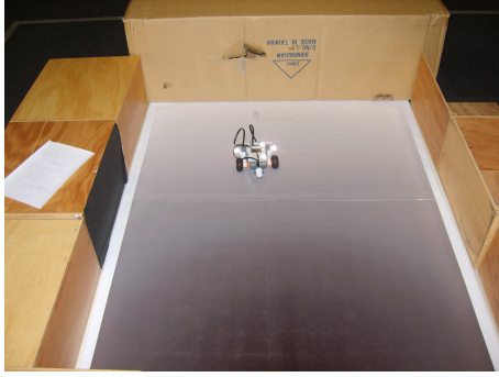
Fig. 2. Lego mindstorm platform in the arena with little background light. The paper in the arena is the simulated pollutant obtained by printing a gradient of black ink on paper. We use the black ink's gradient to simulate a pollutant.
