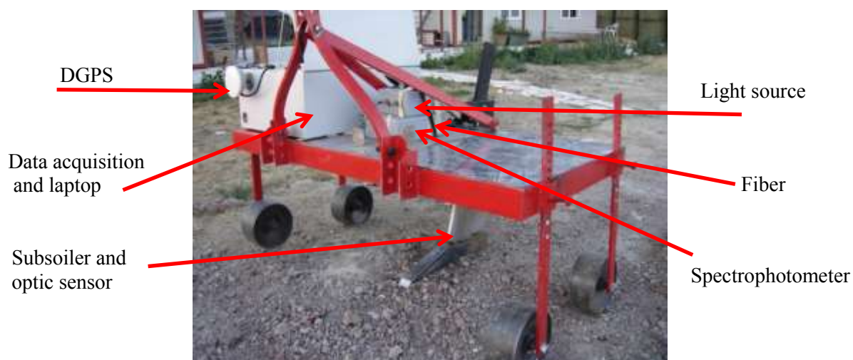
Figure 1. The on-line Vis-Nir soil sensor, as designed by Mouazen [14].
