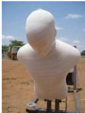
Figure 78: Photograph of the SATS covered with a Mutton cloth layer to test for any penetration effects.
