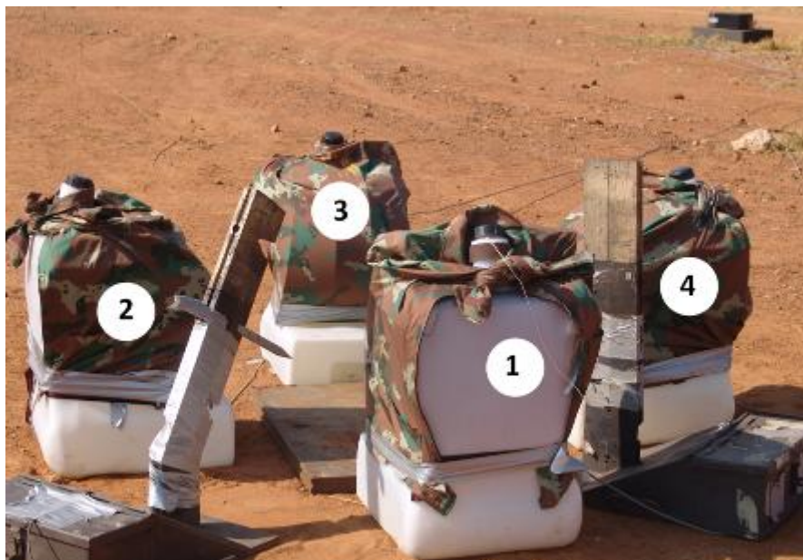
Figure 56: Photograph of the experimental setup of the four SA Waterman torso surrogates and pressure probe prior to the test (1. Foam (50mm thick closed cell polyurethane foam); 2. Lexin; 3. Uniform Only; 4. Aluminium Sheet).
