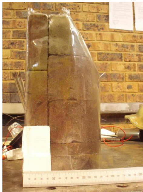
Figure 68: Photograph of the mould created in order to cast the abdominal insert of the SATS.
