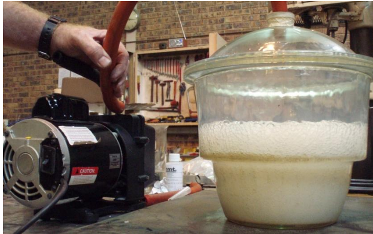
Figure 69: Photograph showing vacuum generated to remove air bubbles from the Dragon Skin™ mixture.
