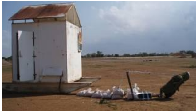
Figure 79: Photograph of the mobile splinter proof shelter in which the data acquisition equipment was placed.
