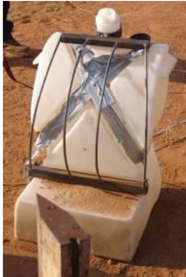
Figure 55: Photograph of a SA Waterman torso surrogate with a bracket mounted on the chest area to protect the chest transducer plate from impact by clothing or PPE.
