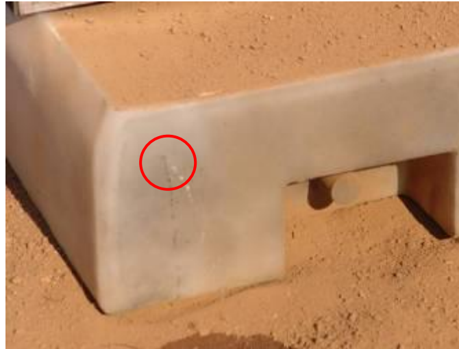
Figure 59: Photograph of the small hole in SA Waterman #4 after the test.
