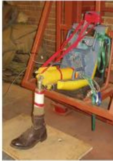
Figure 22: Photograph of the SA Surrogate Leg prior to testing in a vehicle validation test.
