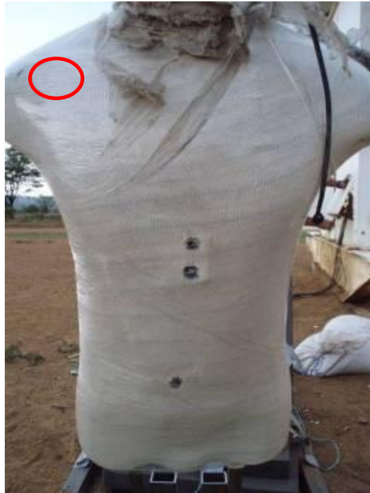
Figure 83: Photograph of the SATS with protective clothing removed to enable the Mutton cloth layer to be inspected for signs of penetrations.
