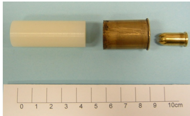
Figure 2 Round Configuration L-R: Dummy round, adaptor, 0.357 Magnum cartridge
