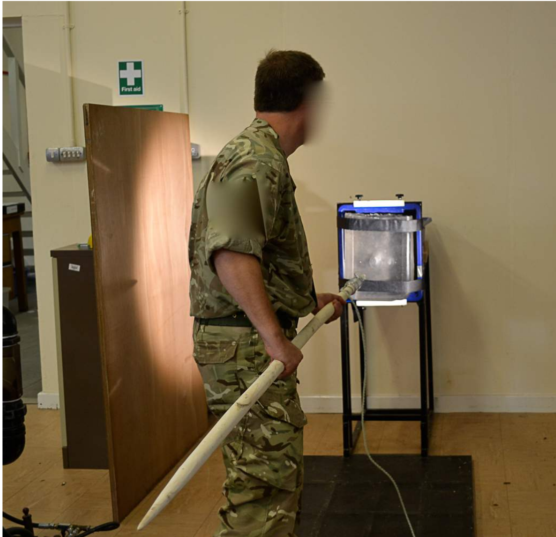
Figure 6: Participant performing spear thrusting in a block of PermaGel™. Hand position was the most typical used by participants.
