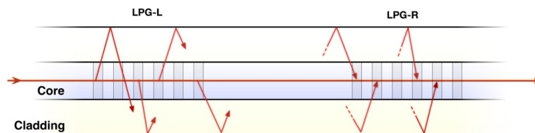
Fig. 7. Schematic of a cascaded LPG sensor showing the left (LPG-L) and right LPGs (LPG-R) and the coupling of the core propagating modes, represented by the arrows, into and out of the cladding.
