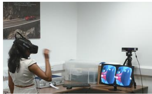
(b) The remote virtual site with a user using an Oculus rift for visualization and Kinect for tracking
