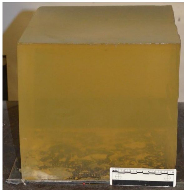
Figure 4-7: 10% gelatine block 250mm in length, cut to size after 5.5mm BB quality control check shot was carried out.
