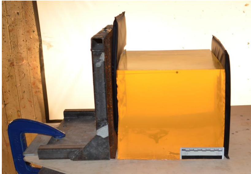
Figure 4-8: Typical target set up of HG2 armour panels on the front and back face of a 10% gelatine block 250mm in length.
