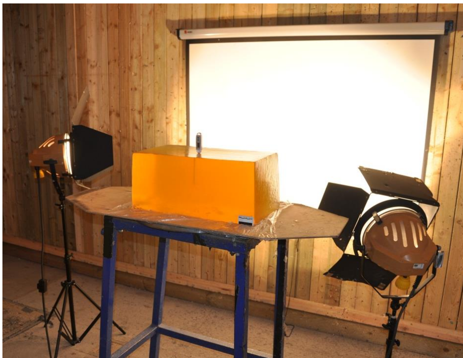
Figure 3-10: Target set up complete with a 20% gelatine block
