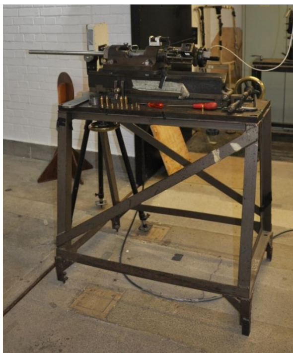
Figure 3-9: Enfield Number 3 Proof Housing set up
