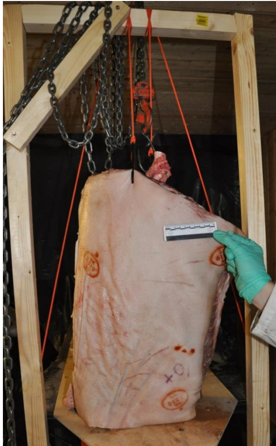
Figure 3-32: View of the typical set up from the front showing the front thoracic wall with the skin facing the muzzle
