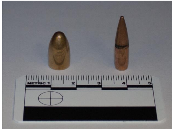
Figure 2-5: A 9mm Luger projectile of mass 7.45 g (left) and an SS109 5.56 x 45mm projectile of mass 4 g (right) for which drag will be calculated throughout this section when the various factors are altered
