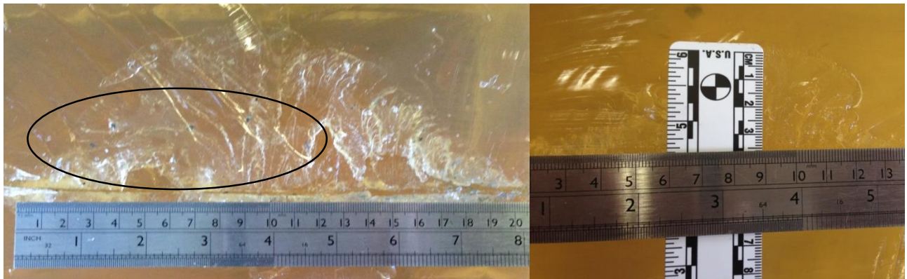
Figure 3-19: Measurement of fissures – length (left) and height measurements (right), with visible debris present highlighted.
