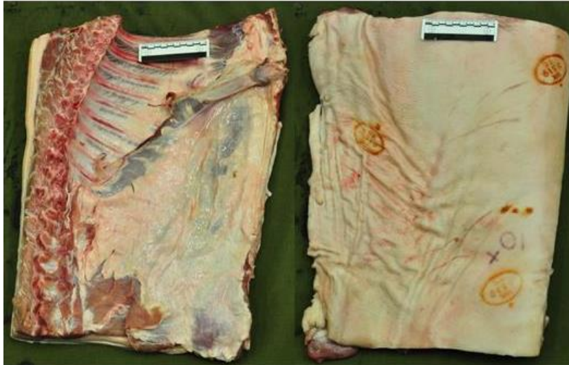
Figure 3-29: A front and back view of a typical example of the porcine thoracic wall tested
