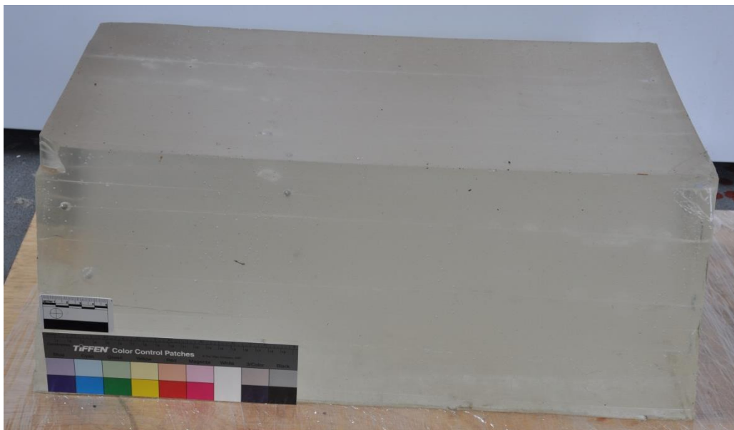
Figure 3-6: Perma-Gel™ block after being re-melted and cast into larger block
