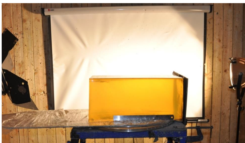
Figure 4-2: Typical target set up of 10% gelatine block 500mm in length with a body armour panel (HG2) on the front face.
