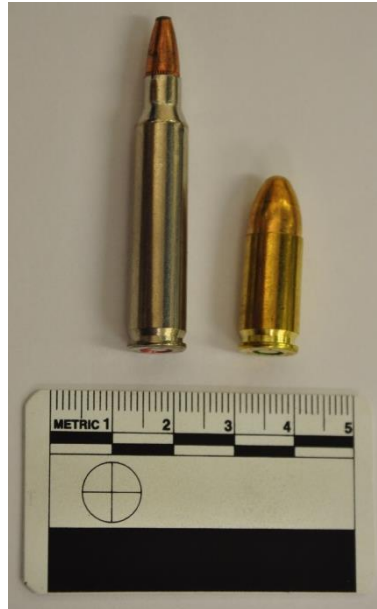
Figure 3-15: A .223 Remington (62 grain; Federal Premium® Tactical® Bonded®)(left) and a 9mm Luger (124 grain; full metal jacket; DM11 A1B2)
