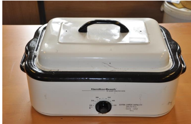
Figure 3-3: Roaster oven used for the melting of Perma-Gel™ raw base media
