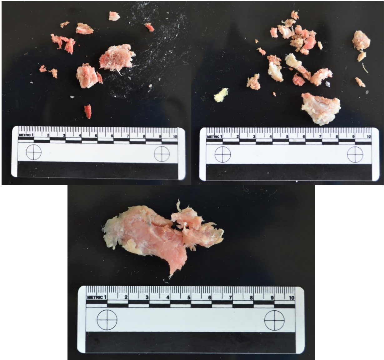
Figure 4-20: Typical tissue debris recovered from 10% gelatine blocks that was situated in between two protected porcine thoracic walls after penetration of a .223 Remington Federal Premium® Tactical® Bonded® round
