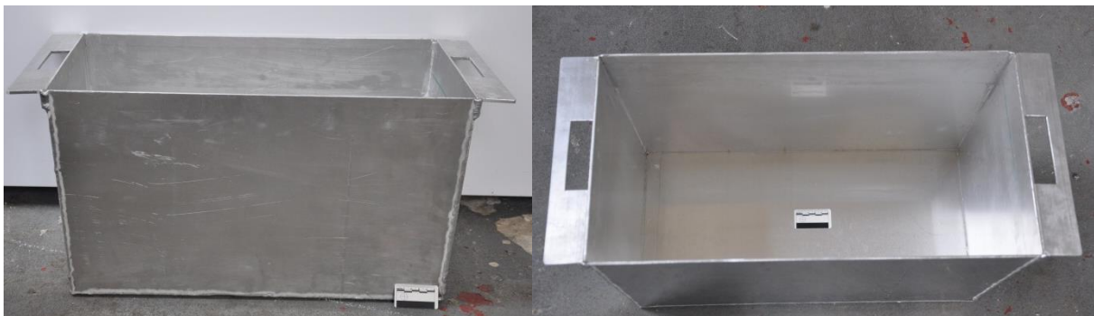
Figure 3-2: Moulds used for casting blocks
