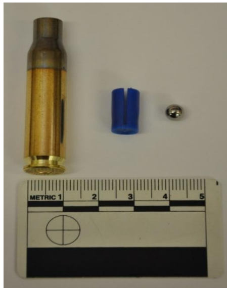
Figure 3-7: 7.56 x 51mm cartridge case, sabot and 5.5mm BB used for DoP testing
