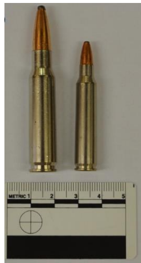
Figure 1. Comparison of both bullet types; (left to right) 7.62mm x 51mm and 5.56mm x 45mm
