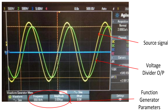
Fig. 15. Test signal of open circuit.
