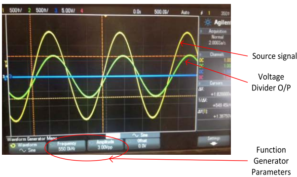
Fig. 16. Test signal for close circuit.
