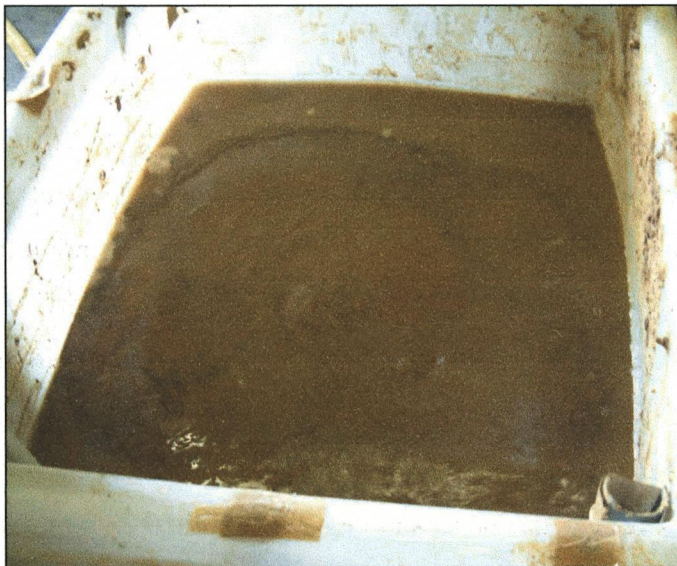
Figure A1.13 First 'sand boil' appearing after one minute
