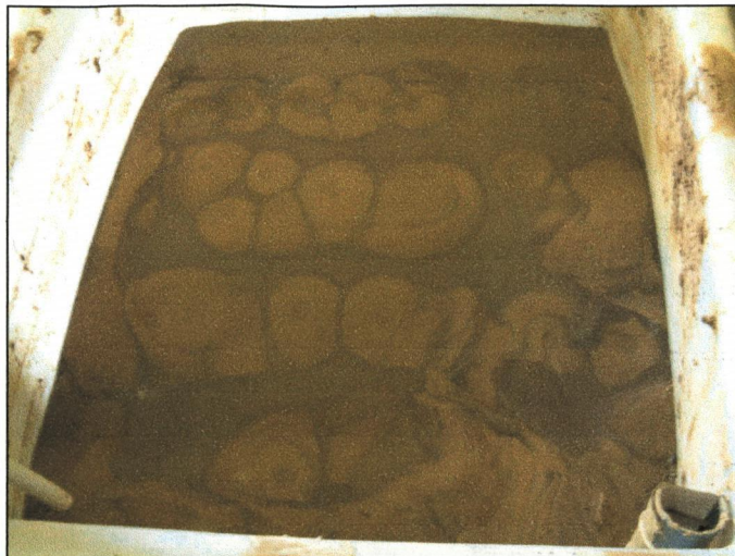
Figure A1.14 Soil surface after upwashing at 0.22 l/s
