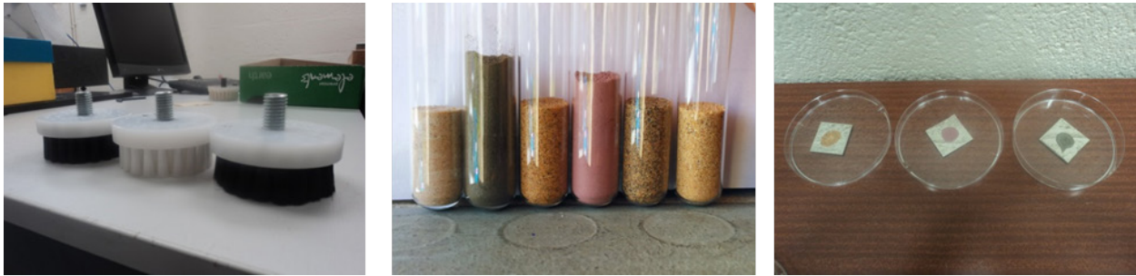
FIGURE 5. Brushes with fixings to Fanuc robot, examples of sand samples, and samples under preparation
