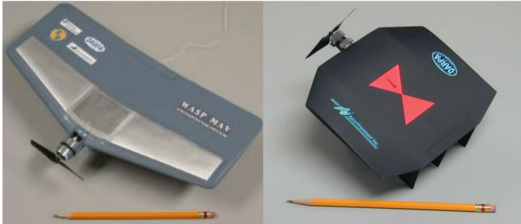
Figure 2-3 Fixed wing Wasp MAV (left) and Black Widow (right) developed by DARPA (Reproduced from internet source).
