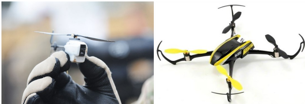
Figure 2-4 Rotary wing Black Hornet developed by Prox Dynamics AS (left); Quadcopter, BLADE NANO QX BNF (right) (Reproduced from internet source).
