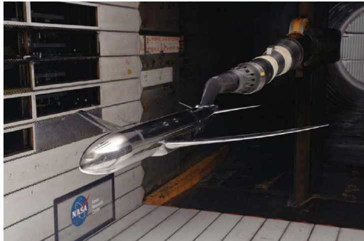
Fig. 3.9 NASA CRM wind tunnel model [18]
