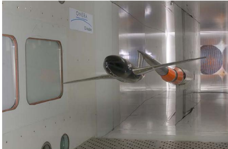
Fig. 3.5 DLR-F6 wind tunnel model [17]
