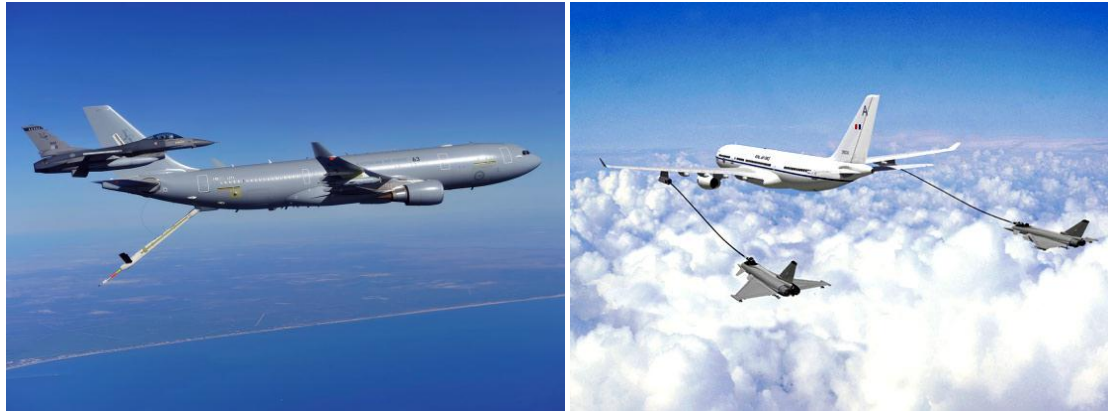
Fig. 2.1 Air-refuelling “flying boom” [14] and “hose-and-drogue” [15] methods.
