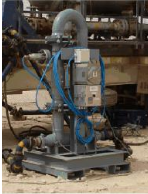
Figure A- 14, Abbon flow Master Optimum C400, taken from Abbon product specification sheet
