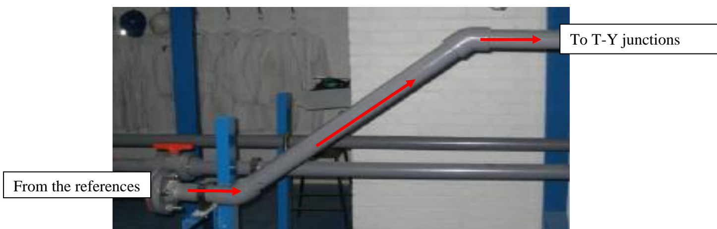
Figure 3-5, The test rig 1m riser
