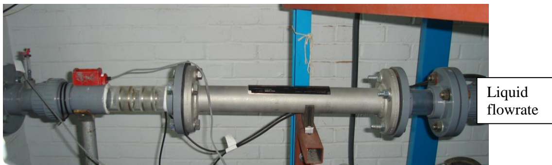
Figure 5-8, Ultrasonic Doppler and static mixer in front of the reference
