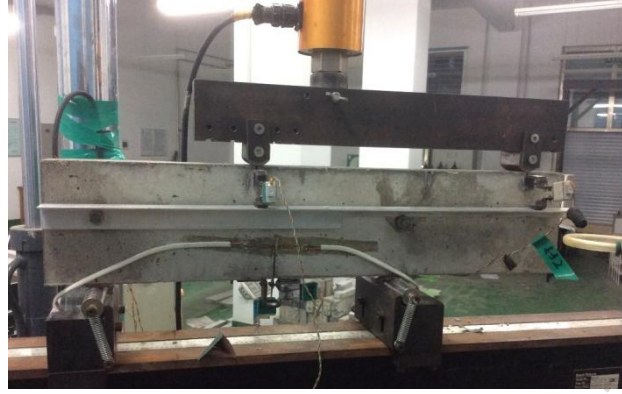
(c) Measurement devices under FPS
