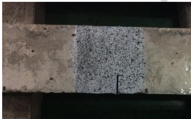
(a) Speckle pattern on specimen surface
