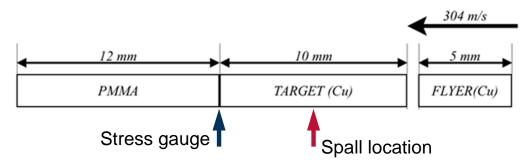
• Axis of flyer and plate is under 1D strain for duration of initial impact and formation of spall plane
