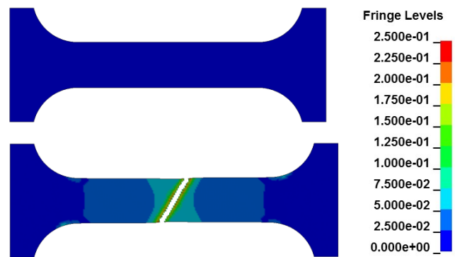
Figure 3: Initial (top) and final (bottom) view of FE tension test model used to check material stress-strain curve. Fringes of effective plastic strain.
