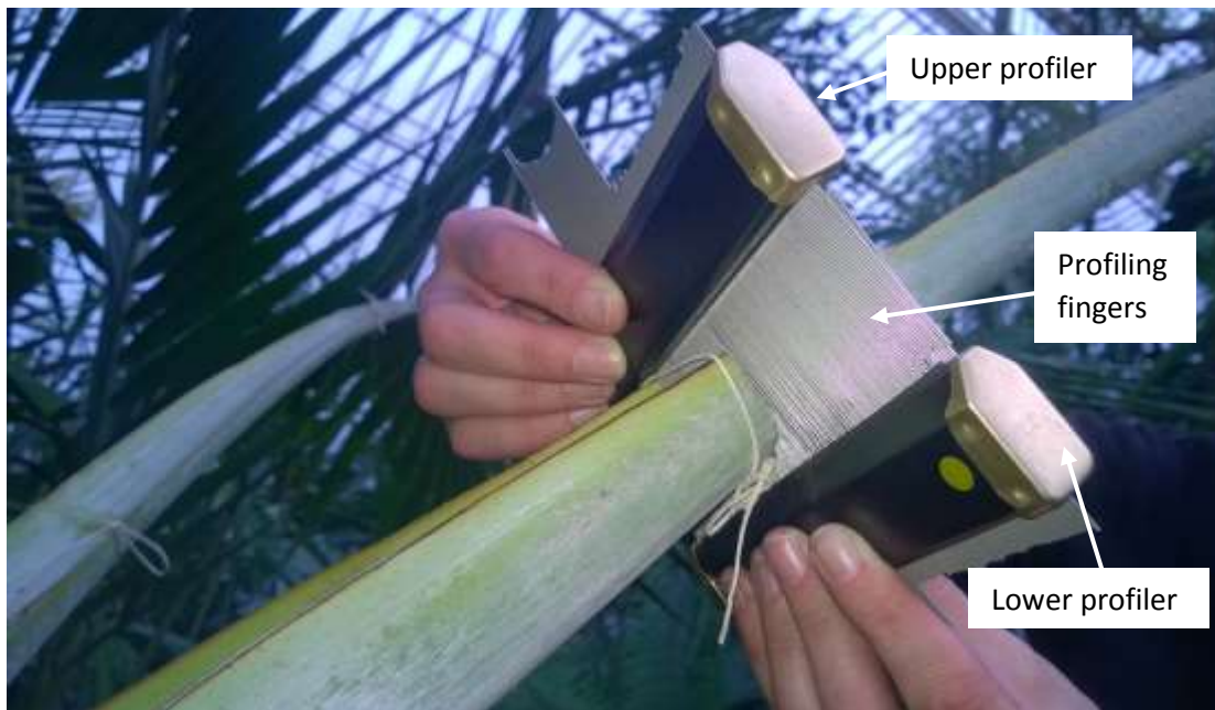
Figure 31 Profiling equipment used to measure the section shape of the petioles
