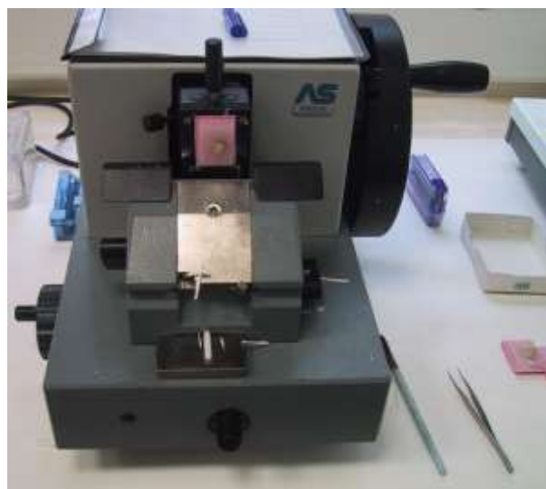
Figure 17 Cutting the petiole sections with a microtome
