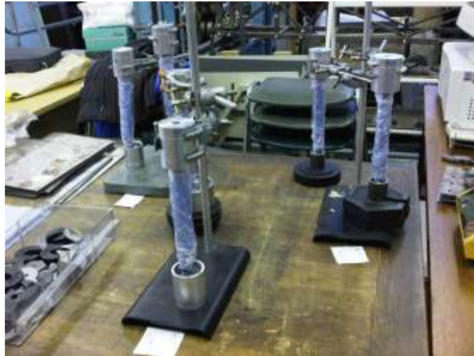
Figure 25 Six petiole segments embedded in epoxy resin and covered in cellulose film prior to torsion testing
