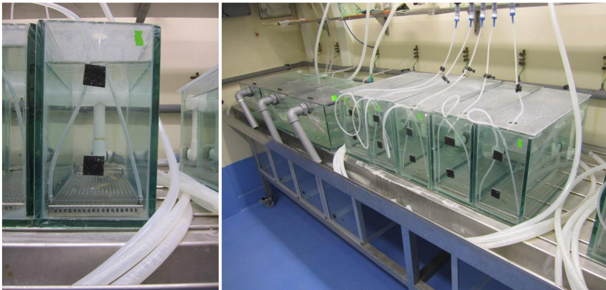
Figure 3.3 The photograph on the left illustrates the narrow breeding tank containing the breeding fish (four females and two males) metal grid, flow-line and air-line. The photograph on the right illustrates five breeding tanks and three holding tanks (one for males and two for females), to enable the breeding females to be rotated to ensure adequate rest days between breeding events.
