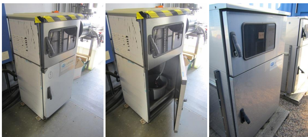
Figure 3.5 Some of the composite samplers positioned along the IPR treatment process. They had to be placed close to an outlet for the specific treatment process, but must not impede access to the containers; therefore, some had to be placed outside the container (as is seen in the far right picture) whereas there was sufficient space for others to be left inside (the left and middle pictures). The middle picture illustrates the collection of the effluent within a glass Winchester.
