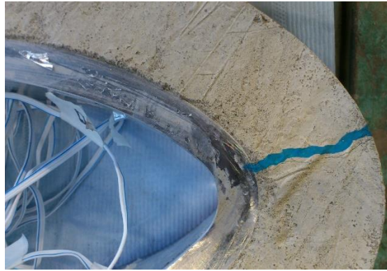
Fig. 6. Crack position in an elliptical ring specimen
