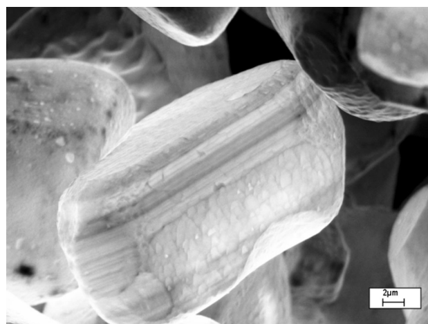
Fig. 3 CL image of ACEL phosphor particles
