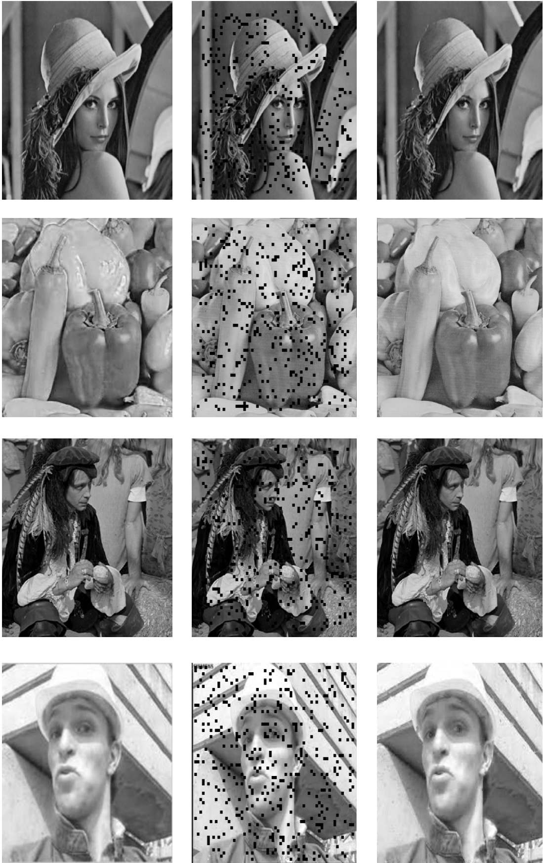
Figure 5.23: From left to right; the original Lena, Peppers, Man and Foreman images, the image with 10% random missing MBs and the restored image.
