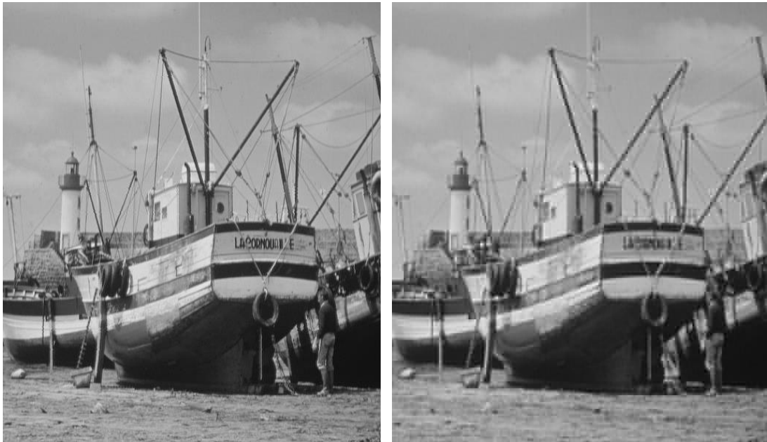
Figure 3.14: Left, original Boat image and right, the reconstructed image using only 7% of the low-frequency 2D-DCT coefficients and applying 2D-IDCT ( 8 \times 8 macro blocks).
