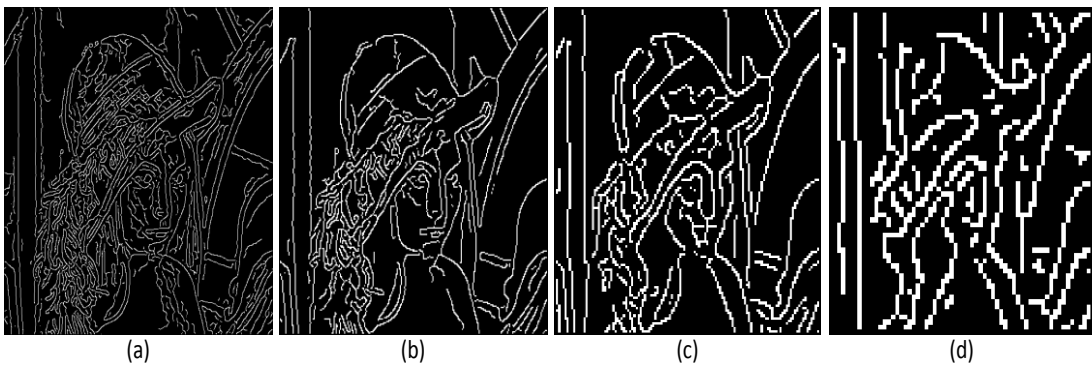
Figure 6.10: Canny edge detector for a multi-scale wavelet on Lena at scales, from left to right: (a) 512^2 ; (b) 256^2 ; (c) 128^2 ; and (d) 64^2 .
