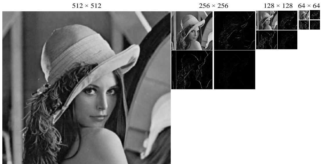
Figure 3.21: Block diagram of the three-stage wavelet pyramid image decomposition and its application to the Lena image.
