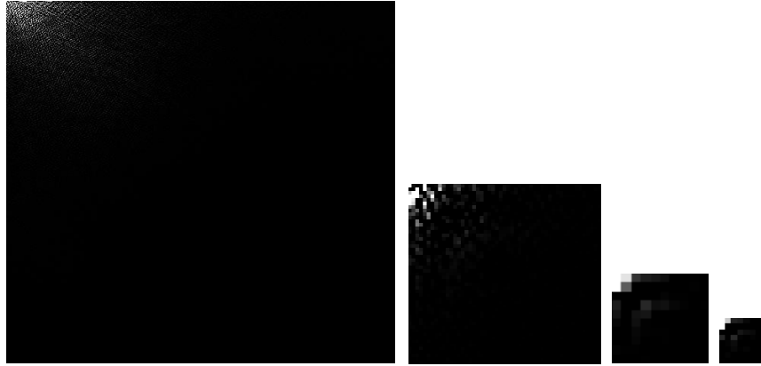
Figure 3.13: From left to right, DCT of Lena image and sub-images of size: (512 \times 512) , (256 \times 256) , (128 \times 128) and (64 \times 64) pixels, respectively.
