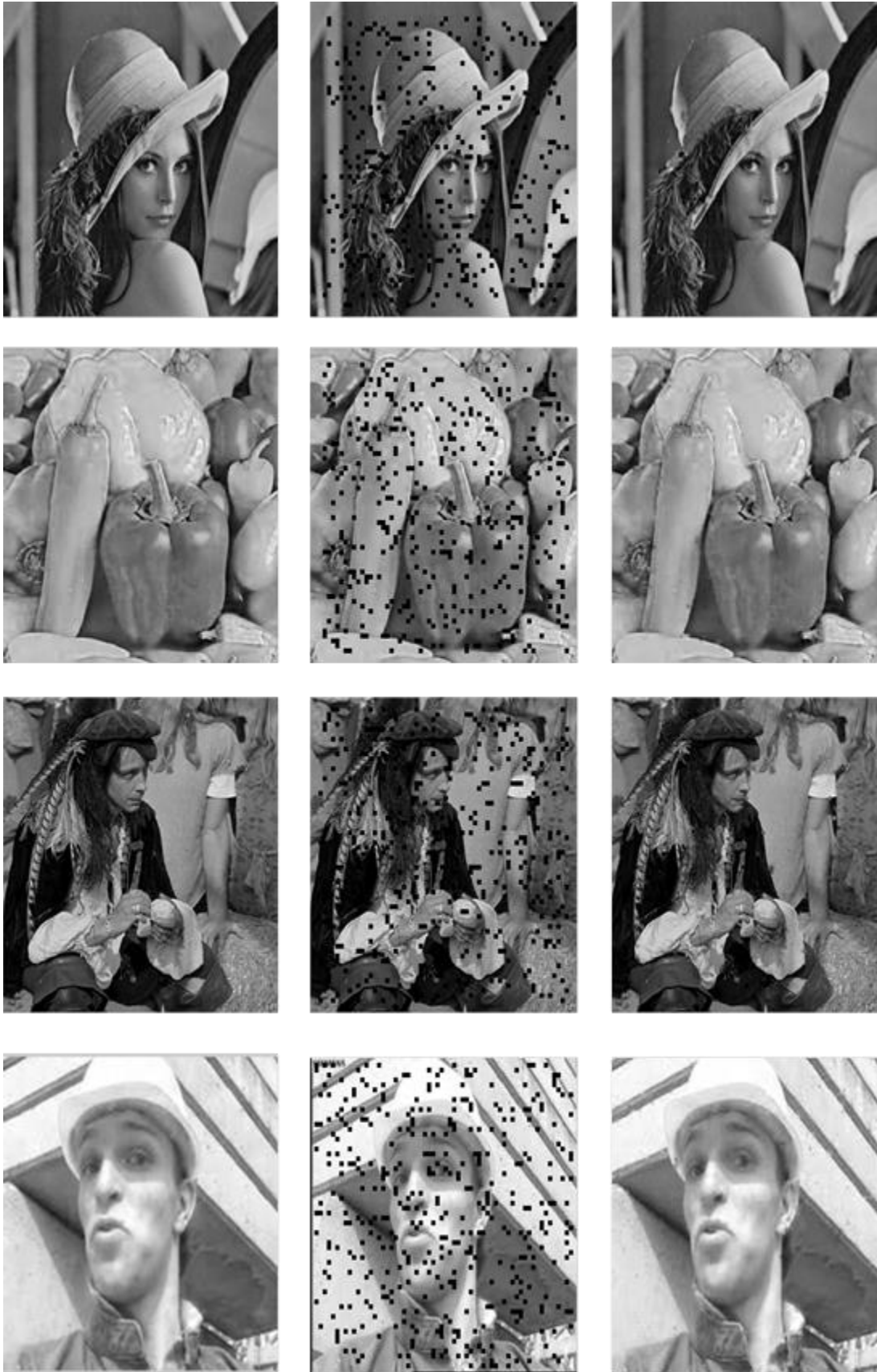
Figure 5.8: From left to right: the original Lena, Peppers, Man and Foreman images, the images with 10% random missing MBs and the restored image for local edge interpolation.
