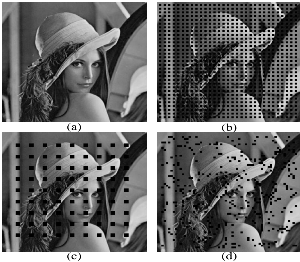
Figure 6.16: (a) original Lena; (b) Lena with 25% macro block loss ( 8 \times 8 ); (c) Lena with macro block loss ( 16 \times 16 ); and (d) Lena with 10% random MB loss ( 8 \times 8 ).
