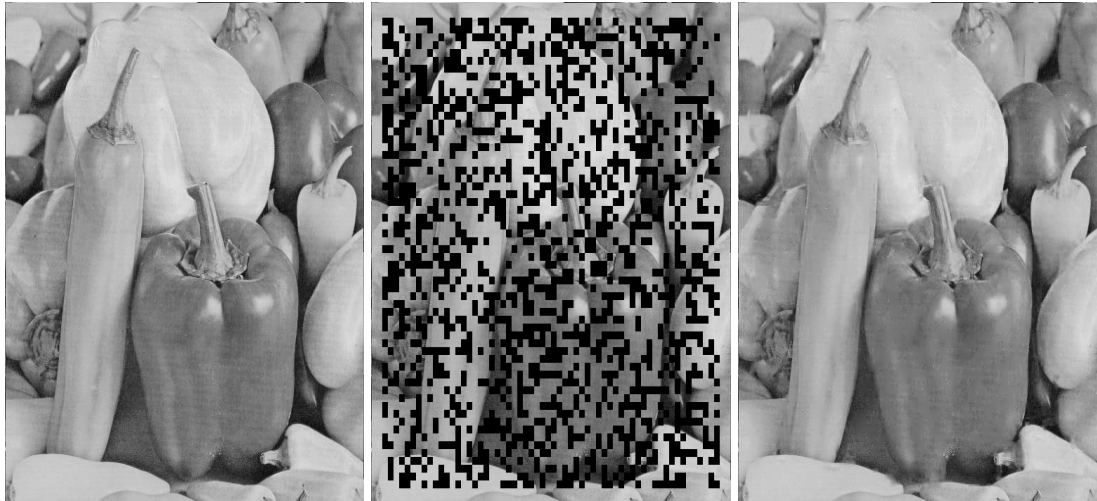
Figure 5.24: From left to right; the original Peppers image, the image with 40% random missing MBs and the restored image.
