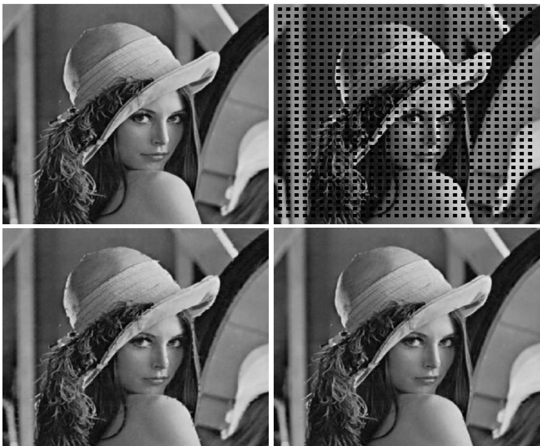
Figure 5.25: Top: from left to right, the original Lena and the image with 25% regular missing MBs (8 \times 8) . Bottom: from left to right, the reconstructed image with local edge-guided interpolation and global edge-guided interpolation.
