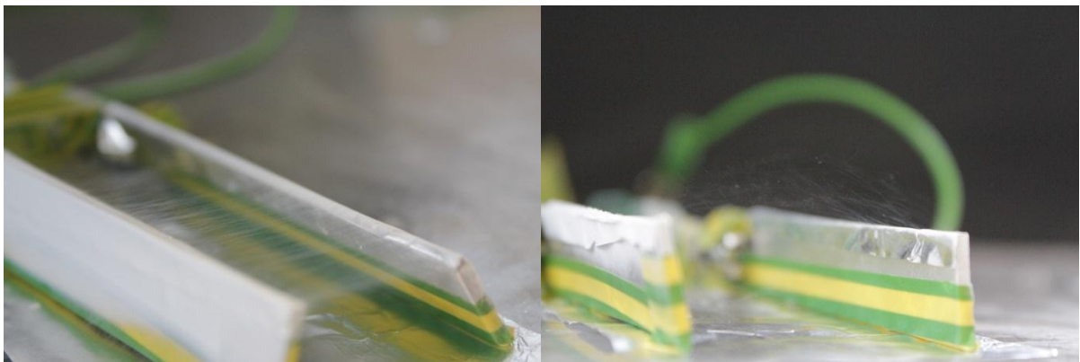
Figure 5.12 - The left image shows aligned fibres between two base electrodes. The right image shows the fibres during electrospinning.
