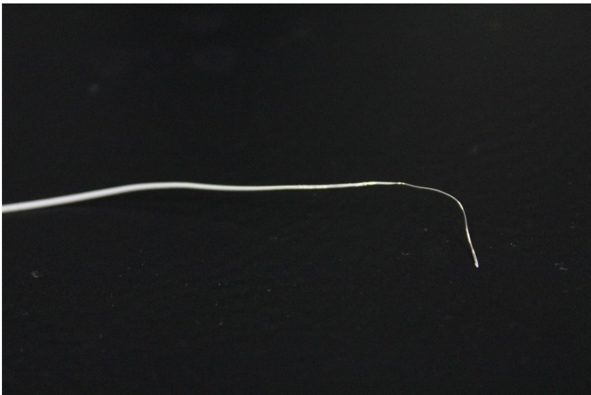
Figure 5.25 - Produced core-shell fibre with the polymer layer thickness decreasing from the left
