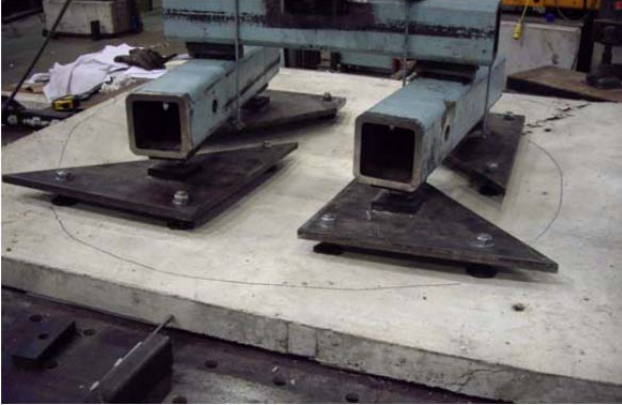
Figure 3: 12-point loading arrangement in the experimental programme [8]
