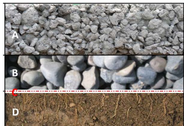
Figure 5. A typical pervious concrete pavement section: A – pervious concrete, B – clean drainage stone, C – nonwoven geotextile, D – underlying soil.
