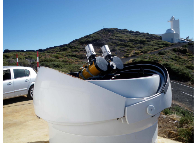
Figure 1. NGTS-P at the Observatorio del Roque de los Muchachos, La Palma, Spain. The prototype initially contained two telescopes but the second camera developed a fault and was returned to the manufacturer shortly after commissioning. All tests described above were carried out with a single camera (iKon1).
