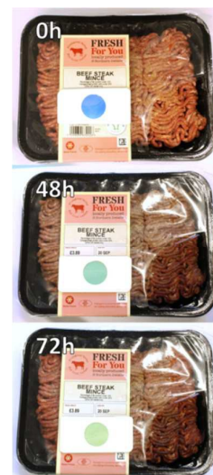
Figure 4 Photographs of an opened package containing beef, refrigerated at 5 °C with the 'consume within' indicator after: 0, 48 and 72 h.
