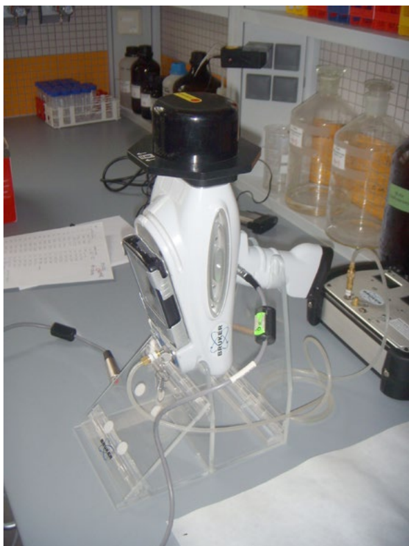
FIGURE 3. THE XRF SPECTROMETER IN THE FACULTY OF CHEMISTRY OF THE ADAM MICKIEWICZ UNIVERSITY IN POZNAŃ (PHOTO: M. KRUEGER).
